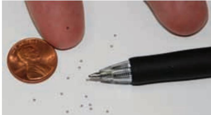
**WCEC will mark copper with almost-invisible microdots, which can easily be detected with a specialized kit that locates the presence of the dots and then allows the reading of ownership information etched on each one.**
