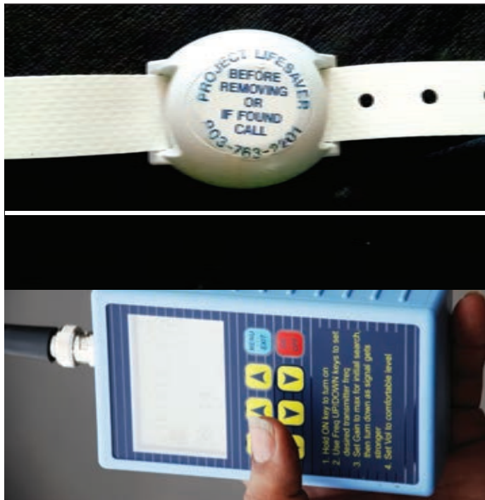
TOP: The bracelets worn by PLI clients are lightweight and waterproof, and have contact information boldly printed. In past instances, this information has sparked an intervention even before a search was begun. BOTTOM: The hand receiver used by the searchers emits sounds that become stronger as the searcher nears the location of a bracelet.
